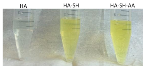
Figure 1. 2,4,6-trinitrobenzene sulfonic acid (TNBS) colorimetric assay for thiol detection on Hyaluronic acid (HA), mono-functional HA with thiol (HA-SH), di-functional HA with thiol and azide (HA-SH-AA).
